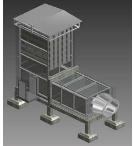
Super Sonic Wind Tunnel Exhaust System, DRDL Hyderabad
